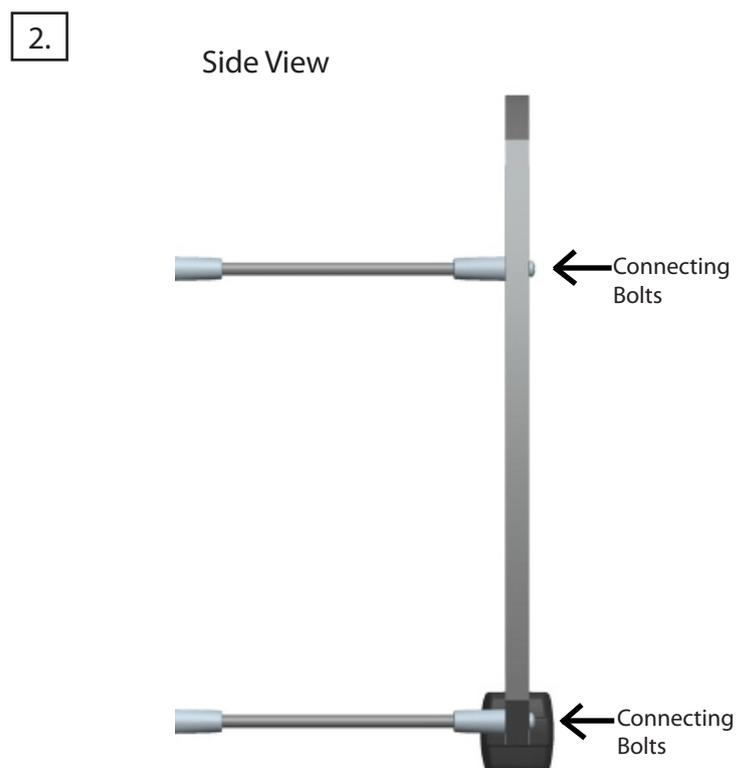
2. Feed the supplied bolts through the 4 holes in the square loop element. Connect the square element to the fiberglass spacers with the bolts and tighten.
