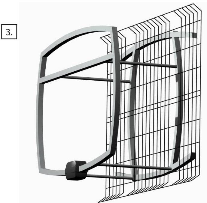
3. Align the separating spacers and attach the reflector (grid) to the spacers by threading the 4 bolts into the spacers. Next attach the 2 "U" Bolt clamps through the holes in the rear frame.
