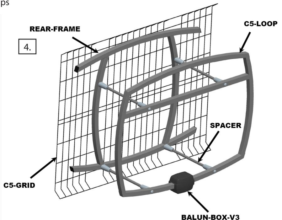
4. **Assembly complete.** Attach the C5 antenna to any kind of mast or mount (up to 2" in diameter) with the adjustable "U" bolt clamps.
